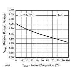
Figure 8. Forward Voltage vs. Ambient Temperature
